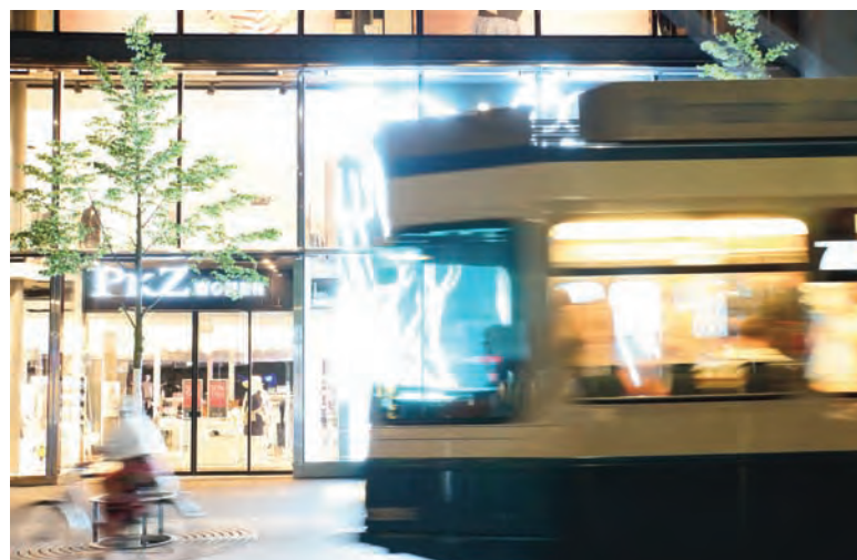
Fig. 8: Tram drivers suffer from the glare caused by the LED installation. Photo: J. Hartmann, July 2015.
